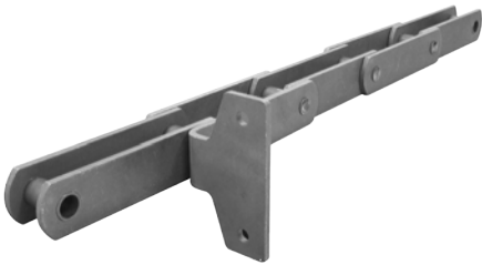
160mm pitch M160 chain with special integral scraper attachment, sheradised plates and Molykote® round parts
