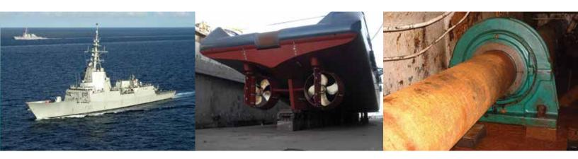
Timken has developed a detailed understanding of the bearing requirements of the marine industry. Part of the program is the innovative split cylindrical roller bearing range; essential components in a marine propulsion drive.
